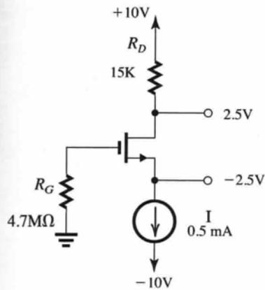
$$V_{GS} = V_t + V_{OV} = 2.5 \text{ V}$$
